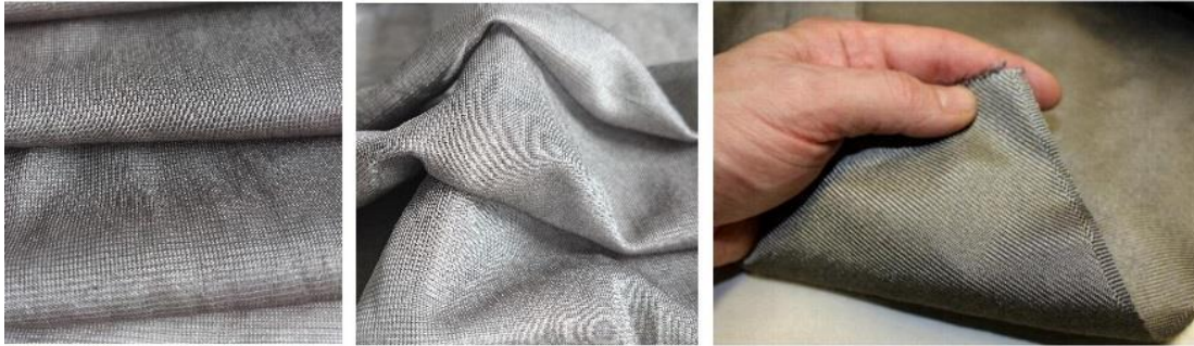
Figure 4: Conductive metalized fabric to cover open parts of the cabinet’s floor.
