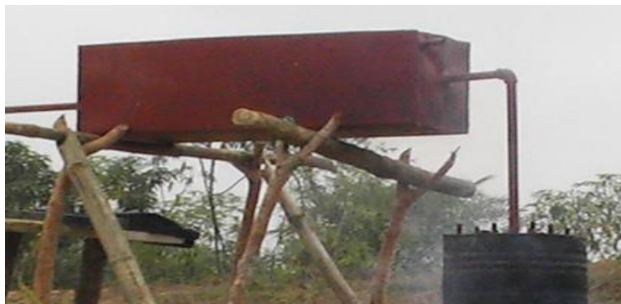
Figure 2: Local equipment for hydrodistillation of essential oils (60 L)
